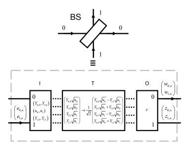
Figure 3. Diagram of a processing unit that performs an ecent-based simulation of a beam splitter (BS). The solid lines represent the input and out channels of the BS. The presence of a message is indicated by arrows on the corresponding channel line. The dashed lines indicate the data flow within the BS.
