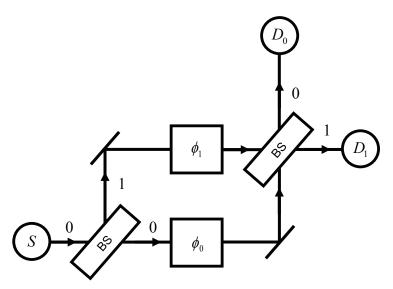
Figure 1. Schematic diagram of the Mach-Zehnder interferometer (MZI) experiment. S: Light source; BS: 50-50 beam splitter;  $\phi_0$ : Phase shifter lower arm;  $\phi_1$ : Phase shifter upper arm; D,  $D_0$ ,  $D_1$ : Detectors.
